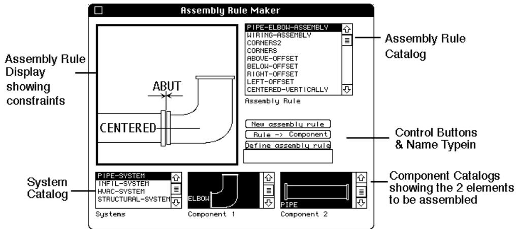
Figure 1. Interface for making assembly rules in Construction Kit Builder (M. D. Gross)
