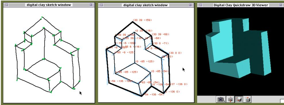
Figure 3. Digital Clay converts freehand sketches into 3D model (E. Schweikardt)
